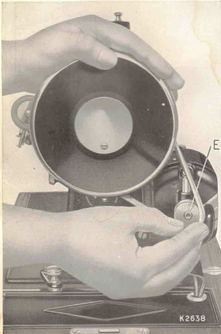
Fig. 4. Springing the Belt into Position.
