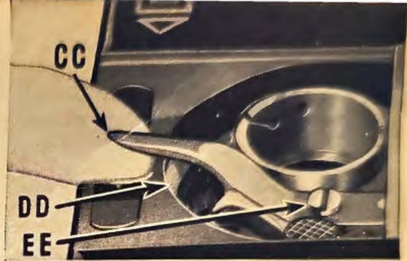
Fig. 32. Raising the Bobbin Case Latch
