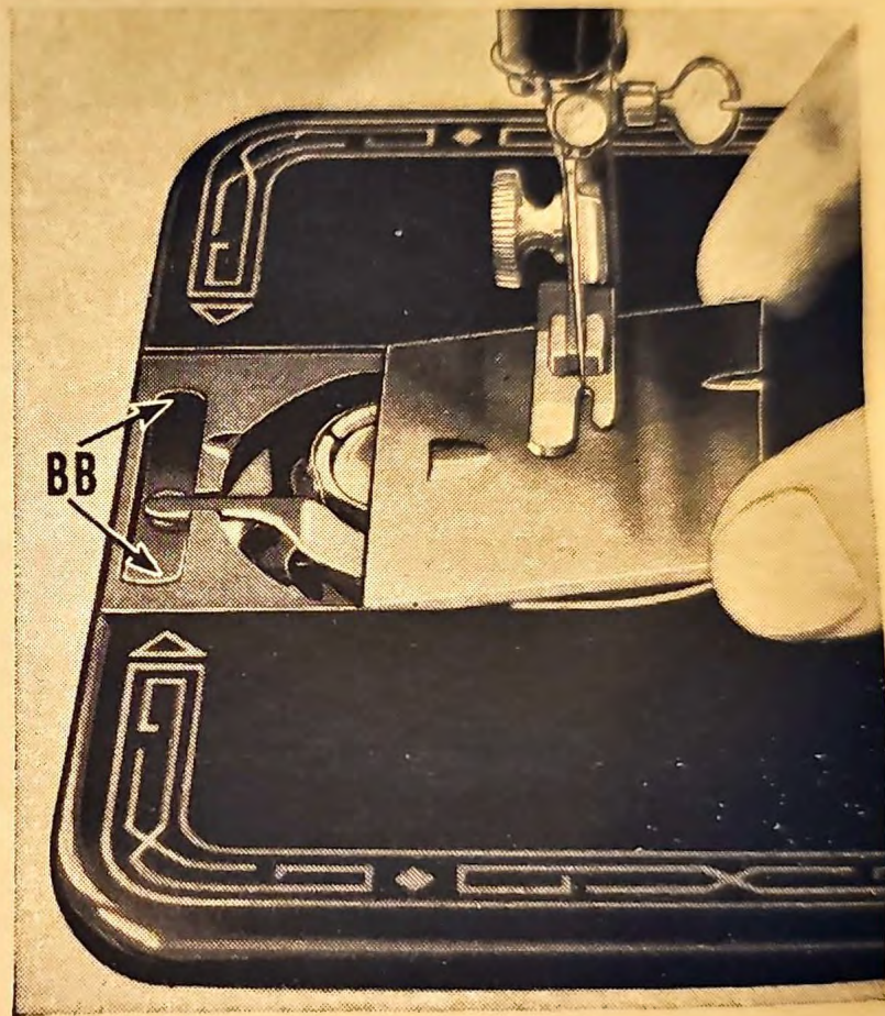
Fig. 35. Replacing the Slide Plate
