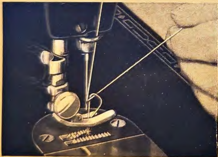
Fig. 17. Drawing Up the Under Thread
