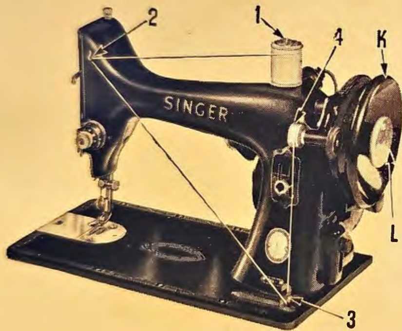
Fig. 11. Machine Threaded for Winding the Bobbin
