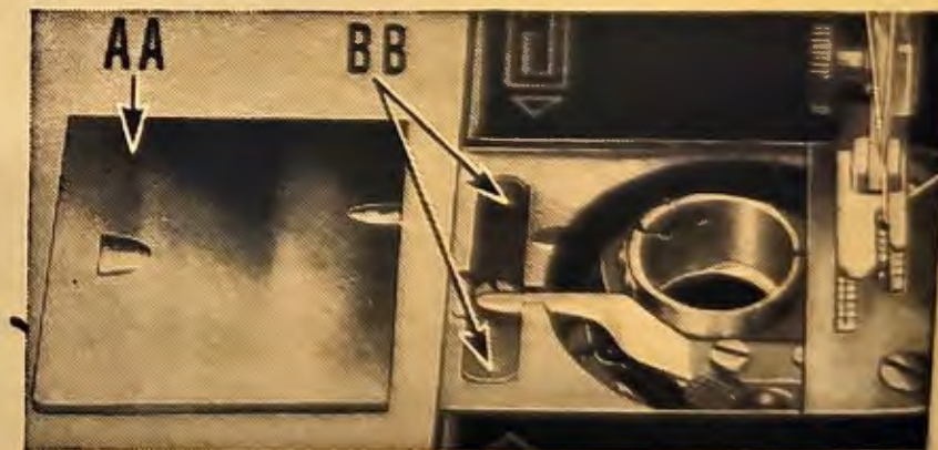
Fig. 31. Slide Plate Removed
