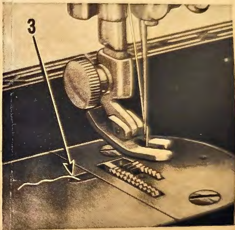
Fig. 16. Under Threading Completed
