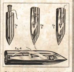
Take the shuttle in the left hand, with the point toward you; draw off about two inches of thread from the bobbin, thread running from the upper side, (see Fig. 1); drop the bobbin into the shuttle as far as it will go; then draw the thread into the open slot of shuttle, at the same time putting a little pressure with 7
