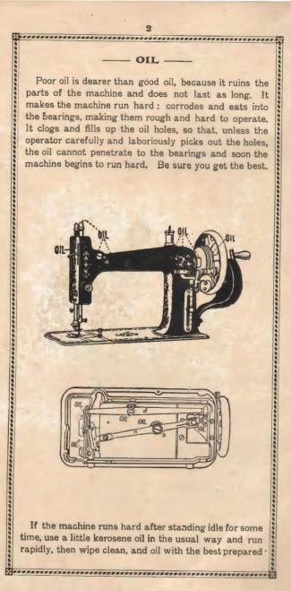
oil. Oil the bobbin-winder in places where there is any friction.
