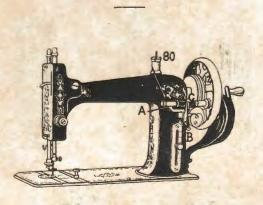
Unlock the balance wheel with thumb and forefinger of the right hand by drawing the key (12) out, turning it part round (this will prevent the machine from wearing, and save the trouble and annoyance of unthreading it, and removing the work while the bobbin is being filled). Then swing the bobbin winder until it is in position and presses firmly against the wheel. Place the spool of thread to be wound from on the spindle (80) and put the bobbin in the bobbin winder. Pass
