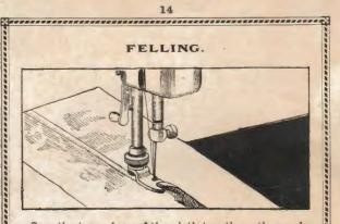
Sew the two edges of the cloth together, the under one projecting one-fourth of an inch beyond the upper; then open out the work and crease the seam down, the wide edge over the narrow edge. Draw the widefolded edge into the hemmer, the same as if it were a hem, and drop the foot. Then guide the fold edge, and work the machine the same as in ordinary hemming. A wider fell requires a wider seam, which is turned the same as a wider hem.
