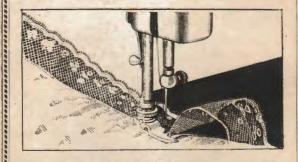
Put the edge of the fabric into the hemmer. When the hem is well started, raise hemmer foot by means of the presser lifter and also raise the needle. Then pass the lace through slot in the side of hemmer, carrying it back under the hemmer on top of the hem. Proceed as in ordinary hemming, keeping lace well in the side.
