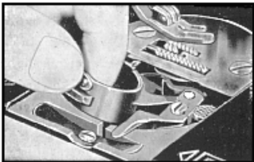
Fig. 33 Removing the Bobbin Case
