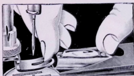
Fig. 8—Removing the shuttle from carrier
