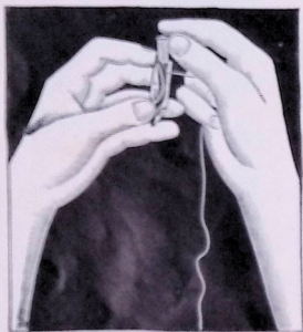
Fig. 9—Starting bobbin in shuttle
