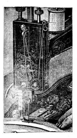
THE STRAIGHT GUIDE is fastened to the plate by a thumbscrew if a seam is to be made parallel to an edge. The straight edge of this guide is fixed so far from the needle that the stitching is formed the desired distance from the edge of the fabric. This guide also serves to sew frills and borders, also to sew in a straight line and at an equal distance from other seams. It saves the trouble of drawing lines.
