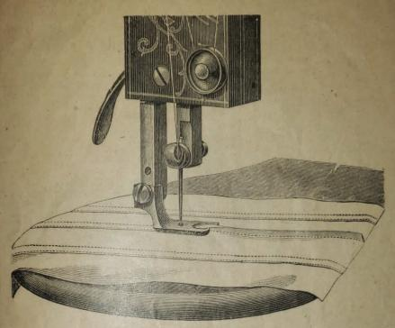
THE FELL-SEAM-FOOT is attached and used similarly to the foregoing hemmer. To make a fell-seam, join the two edges of the fabric by a seam about three eighths of an inch from the edge, then open out the seam, turn one into the hemmer to turn the fell.
