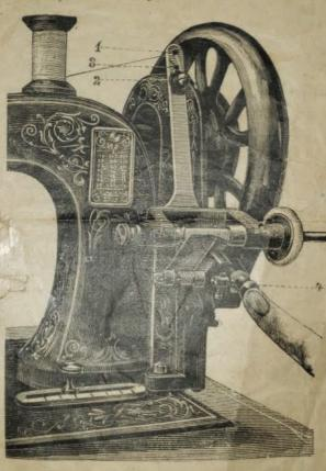
faces you. If the needle be set too high, either the shuttle cannot pass through the loop, or it will not enter the loop freely, and the thread will be cut. If the needle be set too low, the loop will be too large and twist, the shuttle will then occasionally miss it, and stitches will be dropped. It is most important to set the needle correctly.
