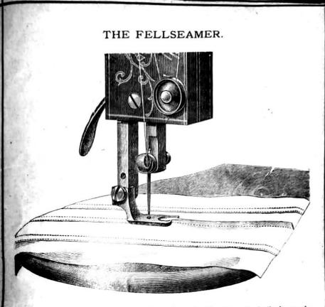
THE FELL-SEAM-FOOT is attached and used similarly to the foregoing hemmer. To make a fell-seam, join the two edges of the fabric by a seam about three eighths of an inch from the edge, then open out the seam, turn one into the hemmer to turn the fell.
