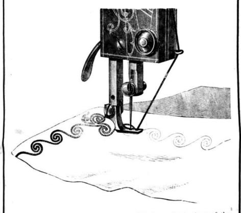
THE BRAIDER is a presser-foot which has a slot in front of the needle hole. It is to be attached to the presser-bar. A wooden spool upon which the braid is evenly wound is placed upon one of the pins. The end of the braid is passed through the eyelet, then through the slot in the braider and drawn back, so that it lies right under the needle. It is only necessary to guide the fabric properly to sew down the braid to any previously designed pattern.
