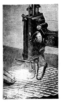
THE QUILTING GUIDE. Attach the guide as shown by the engraving, make a straight line upon the fabric with chalk or by creasing, and stitch upon it; then adjust the gauge-arm to the required distance for the next line of stitching, and guide the fabric with the line already sewn directly under the gauge-arm. This second line serves in like manner as a guide for the third and so on.
