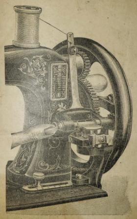
on the right in the end of the knife blade (1), under and between the tension discs (2), then through the slit on the left (3), from thence behind the knife blade down to the bobbin and from inwards to outwards through the small hole in the right hand brass flange and fasten the thread by squeezing it between the flange and the spindle; then wind up all the slack thread by turning the reel on the pin.
