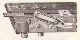
7. TO REMOVE THE SHUTTLE. Bring the Needle bar to its lowest position, pull out the sliding plate No. 77 slowly and the shuttle will rise out of the race.
