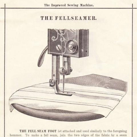
**THE FELL SEAM FOOT** ist attached and used similarly to the foregoing hemmer. To make a fell seam, join the two edges of the fabric by a seam about three eighths of an inch from the edge, then open out the seam, turn one into the hemmer to turn the fell.
