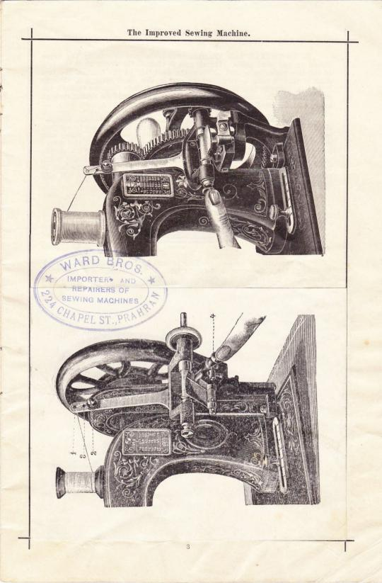
5. TO THREAD THE NEEDLE. Place the reel containing the upper thread on one of the pins. Thence pass it through the eyelet 29 at the side of the face plate, under and between the discs (18) on the front of the face plate so that it runs upwards; to the eye in the check lever (33), through it, and through the hole in the needle clamp, and lastly *from you* through the eye of the needle. About four inches of thread should be drawn through the eye of the needle.
