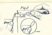
Hold the threader up-side-down with the hook at the top, as shown in Fig. 2. Straddle the needle with the jaws of the hook guard and push the threader hook through the eye of the needle as far as it will go.
