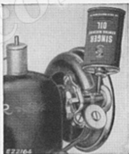
Fig. 30. Oiling the Bobbin Winder
