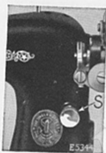
Fig. 22. Stitch Regulating Screw on SINGER 66-4, 99-13, 127 and 128 Machines
