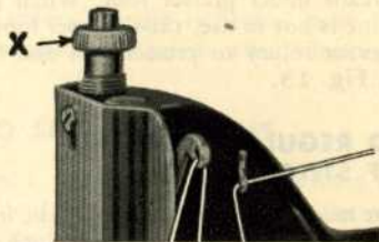
Fig. 15. Thumb Screw for Regulating Pressure on Presser Foot
