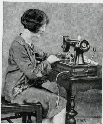
FIG. 13. KNEE LEVER IN POSITION READY FOR OPERATION ON PORTABLE SET 204 ALSO ELECTRICAL CONNECTION
