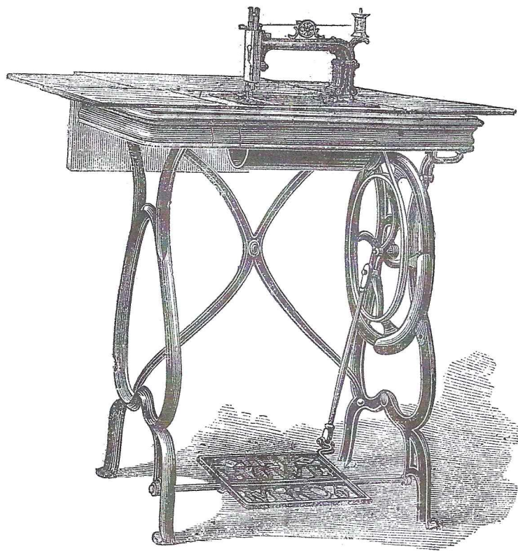
Figure 2-99. Howe (Stockwell Brothers). This stand had a cover which unfolded to create more work area (F/2).
