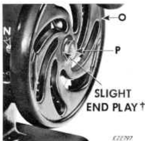
Fig. 16. Adjusting for End Play of Hand Wheel
