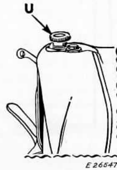
Fig. 22 Thumb Screw for Adjusting Pressure
